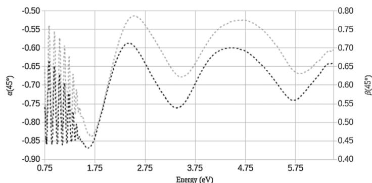
Determining the thickness is straightforward for large enough thicknesses (allowing for clear interference fringes) but becomes tricky for very thin layers (a few nm). This also implies that it will be more difficult to determine the thickness for very absorbing materials, where the light penetration depth is short. In that case, one may use the fact that interference fringes shift to longer wavelengths with increasing wavelength and build a calibration curve using samples of known thicknesses.
